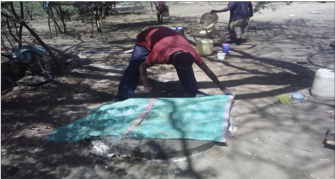
2. SANPLAT Slabs being manufactured for vulnerable community members households for improved sanitation
